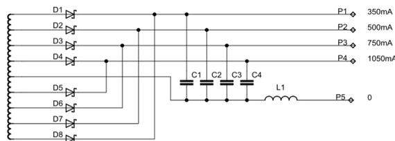
Figure 4: Multiple transformer tapings and multiple outputs
