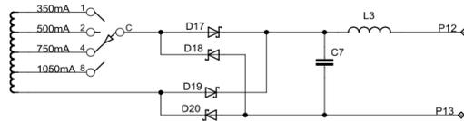
Figure 3: Switchable outputs
