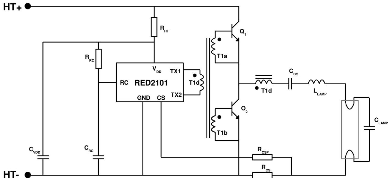
Figure 3: RED2101 Application diagram
