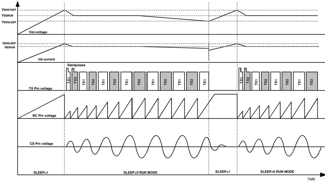
Figure 4: RED2101 Startup waveforms
