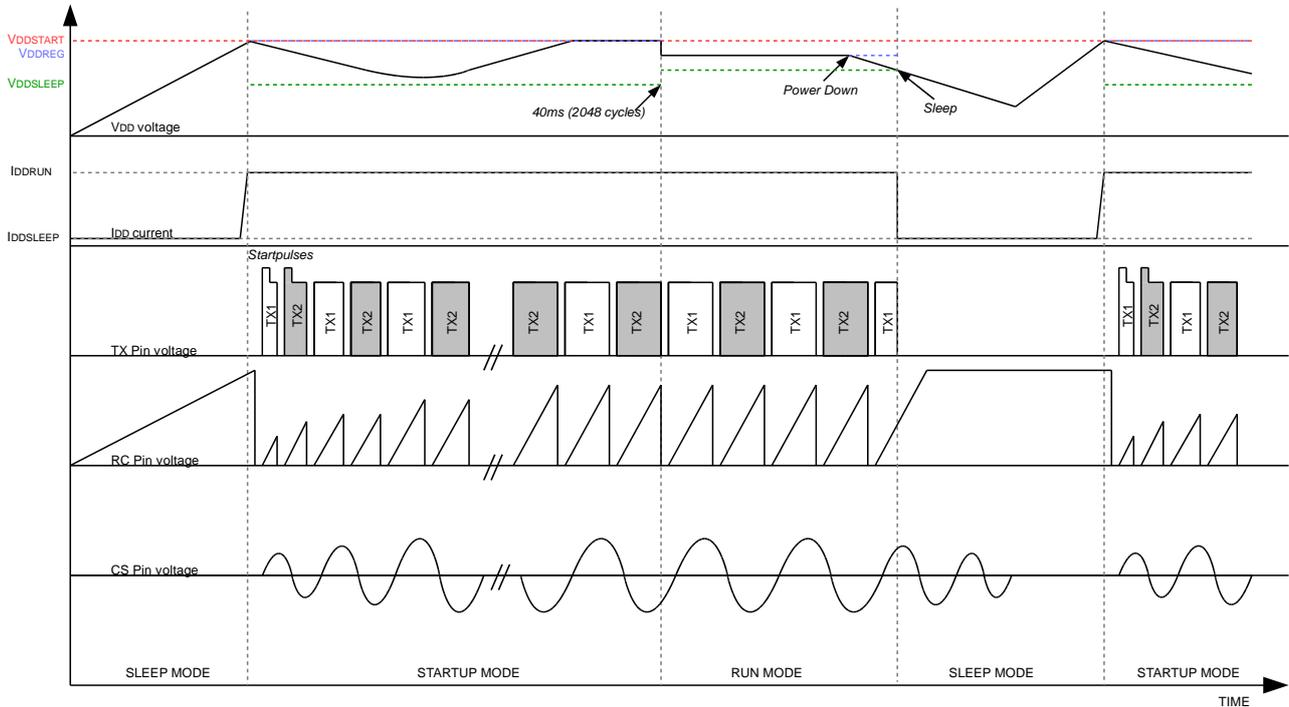
Figure 4: IC Start-up waveforms
