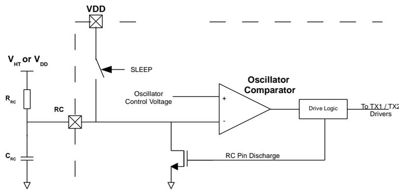
Figure 8: Oscillator circuit
