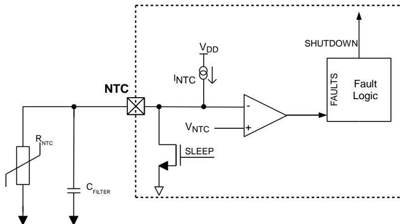
Figure 9: RED2541 NTC pin circuit
