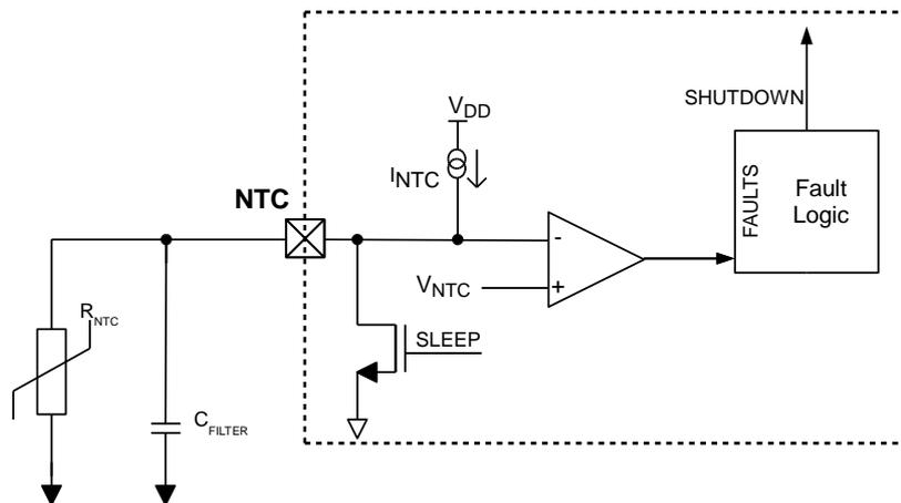
Figure 9: RED2541 NTC pin circuit
