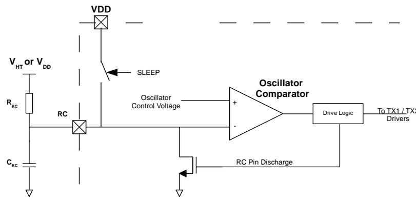
Figure 8: Oscillator circuit
