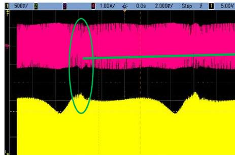
Figure 10: Primary current and RC pin on edge of capacitive mode switching
