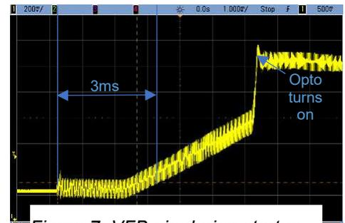
Figure 7: VFB pin during startup
