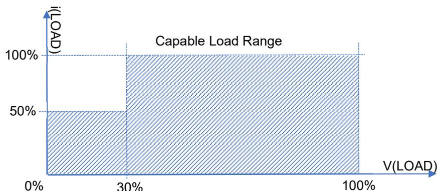
Figure 5: Static characteristics of allowed loads
