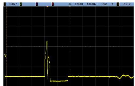
Figure 3: Tx pin drive pulse
